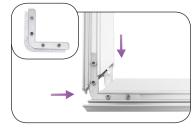
**a.** Corner Connector: Align front lock plate with back pressure plate, back-to-back.
