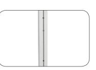
**d.** *Note:* Side extrusions will have holes toward bottom for feet type: Yeti or Aspen Side Feet.
