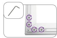
**c.** Then slide adajacent extrusion onto the Corner Connector.
