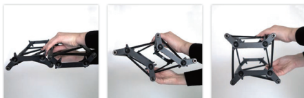
Unfolding of Truss module
